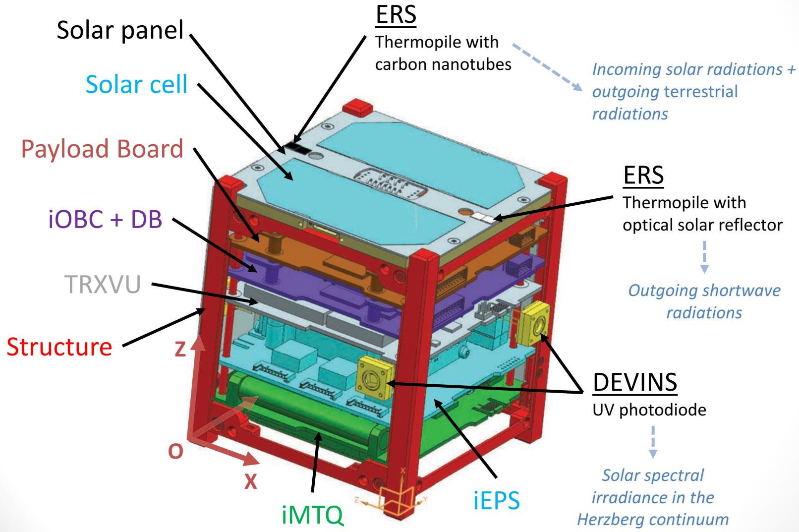
→ Payload Sensors with broad bands Field of View
